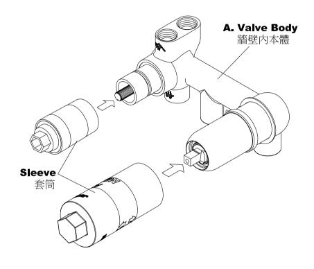
\* Use **Sleeves** to protect the cartridge and thread before installation, and **Sleeves** could be removed only after complete the finished wall. 使用套筒保護陶瓷中心栓及螺牙,必須在安裝程序前先套上。完成 埋壁體安裝程序後才可以取下套筒。
