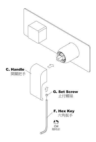
\* Assemble the **Handle** to **Spindle of Cartridge**, and then tighten the **Set Screw** with **Hex Key**.
