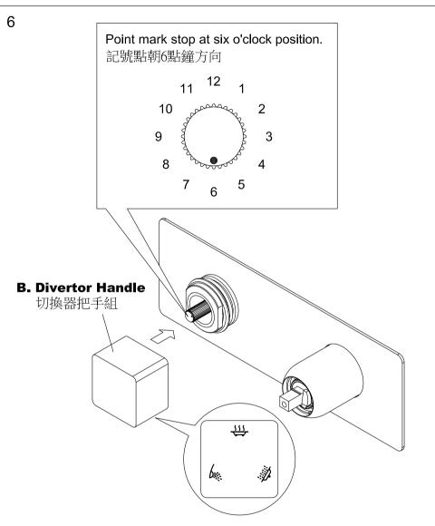
\* Face to the main body, and then turn the **Divertor Spindle** until the point mark stop at six o'clock position. Press **Divertor Handle** onto valve spindle until heard a click sound.
