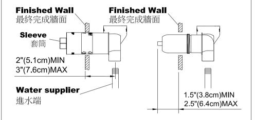
\* Connect hot and cold supply pipes to the **Valve Body**, and keep the distance between 2" (5.1cm) minimum and 3" (7.6cm) maximum from the Finished Wall to the center of **Valve Body**; or keep the distance be 1.5 " (3.8cm) to 2.5" (6.4cm) between top of cartridge and Finished Wall for necessary conditions.
