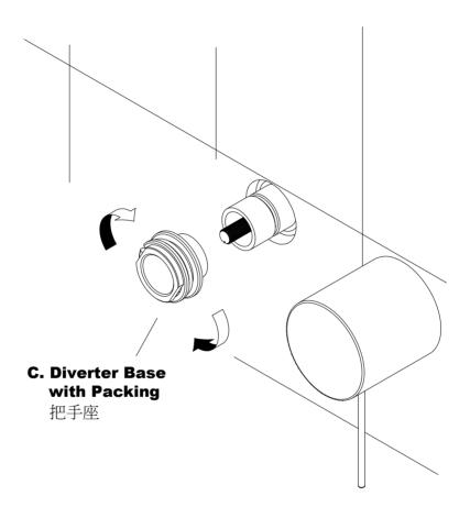
\* Screw in the Diverter Base as shown on Figure above.
