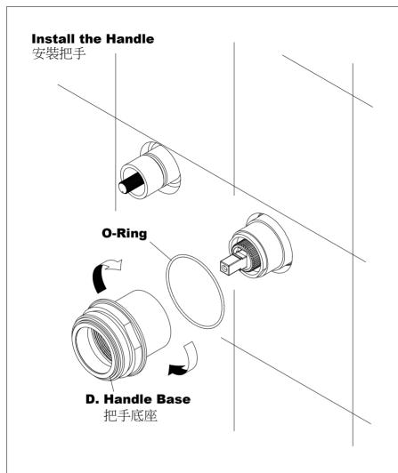
\* Screw in the **Handle Base** with **O-Ring** clockwise to the **Valve Body** and tighten it. Please notice the **O-Ring** has to be placed between base and wall.
