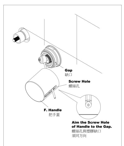
\* Insert the Lever through a hole in the **Handle**. Completely cover the handle base. Aim the screw hole into the gap.
