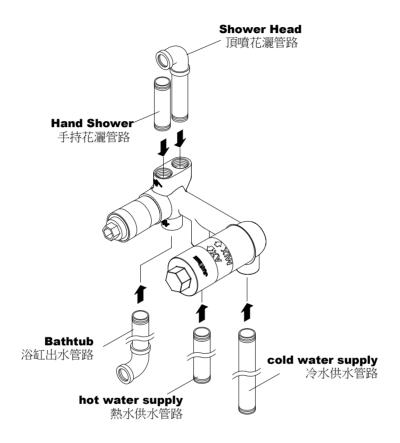
\* Install outlet pipes, hot and cold water supply pipes as figure shows. 依圖示,安裝冷熱供水管路以及浴缸、手持、頂噴花灑管路。
