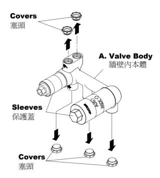
\* Use **Sleeves** to protect the cartridge and thread before installation, **Sleeves** shall only be removed after finishing the wall.
