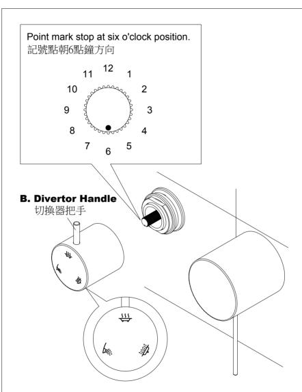
\* Turn the **Divertor Spindle** until the point mark stops at 6 o'clock position. Insert **Divertor Handle** into the spindle. You shall hear a "click" sound.
