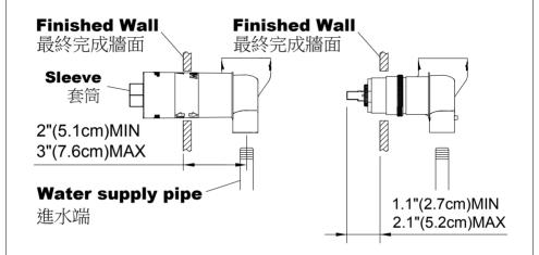
\* Connect hot and cold supplies pipes to the valve body, keep the distance between 2"(5.1cm) minimum and 3"(7.6cm) maximum from the finished wall; or keep the distance from 1.1" (2.7cm) to 2.1" (5.2cm) between top of cartridge and **Finished Wall** for necessary conditions.
