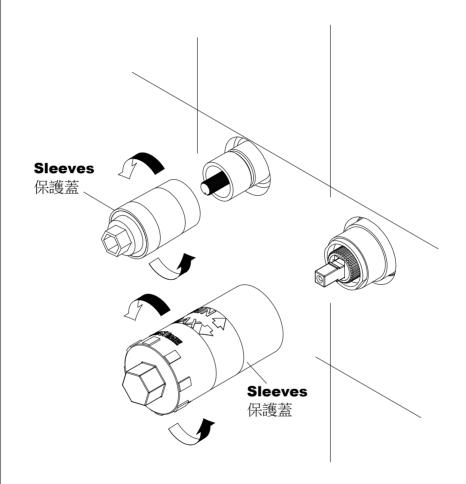
\* Remove the **Sleeves** only when the proper **Lever** was selected. 確認適用的把手桿後,再將保護蓋卸除,進行後續組裝。
